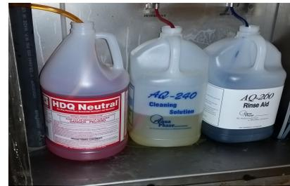
1. Place Chemical Solutions in the Chemical Tray (located inside the Chemical Cabinet at the rear of the Aqua Phase) as the locations marked "**DETERGENT**" and "**RINSE-AID**".
