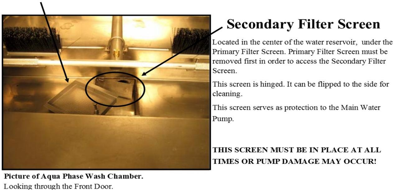
**IF YOUR UNIT DOES NOT HAVE THE FILTER SCREENS SEATED PROPERLY, IN THEIR PLACE AT ALL TIMES, YOU CAN EXPECT THE SPRAY NOZZLES TO BECOME CLOGGED.**
